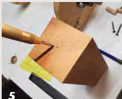
5 Mark the center at the ends of the spindles, and drill ½"-diameter holes to accept the pivot dowels.
