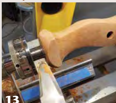
13 Each leg is mounted individually on the lathe, now on its true center, so the foot profile can be formed.
